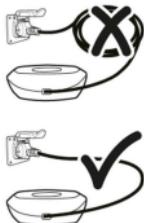
The electrical lead must always be fully unrolled before it is connected to a power socket.
